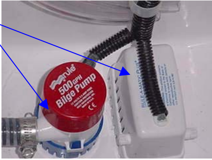
Aft bilge pump and float switch are located in the aft bilge area
