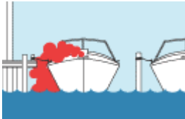
Blocked exhaust outlets.
