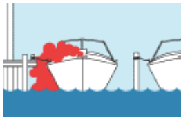
Blocked exhaust outlets.
