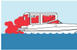
Inadequately ventilated canvas enclosures.
