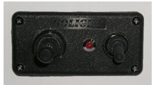
Remote spot light control panel
