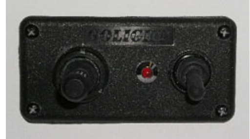
Remote spot light control panel
