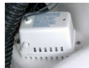
The high water float switch is located further aft on the port side of the bilge.
