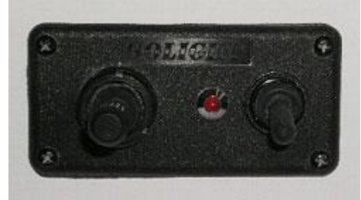
Remote spot light control panel
