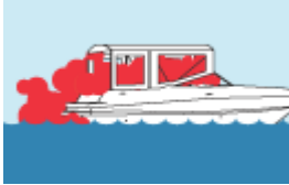
Inadequately ventilated canvas enclosures.
