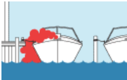
Blocked exhaust outlets.
