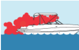
Exhaust gas trapped in enclosed places.
