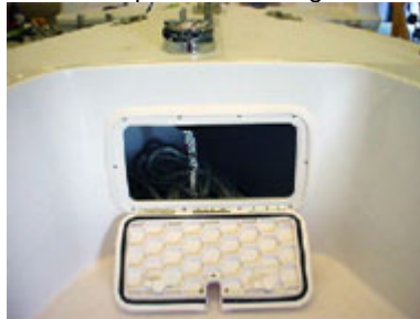
Rope locker storage
