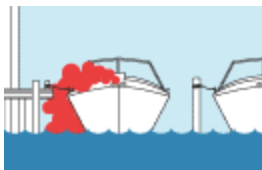
Blocked exhaust outlets.
