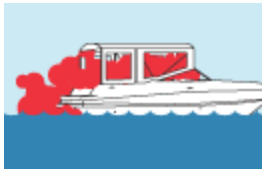
Inadequately ventilated canvas enclosures.
