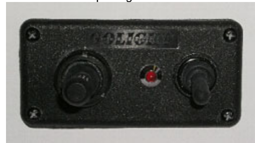
Remote Spot Light Control Panel
