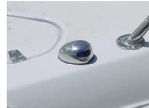
The U.S. Coast Guard requires that the anchor/all around light be installed at the highest point on the boat and must be secured in the up position when you are underway. Therefore, this light will be installed as follows based upon the optional top that you may have selected:
