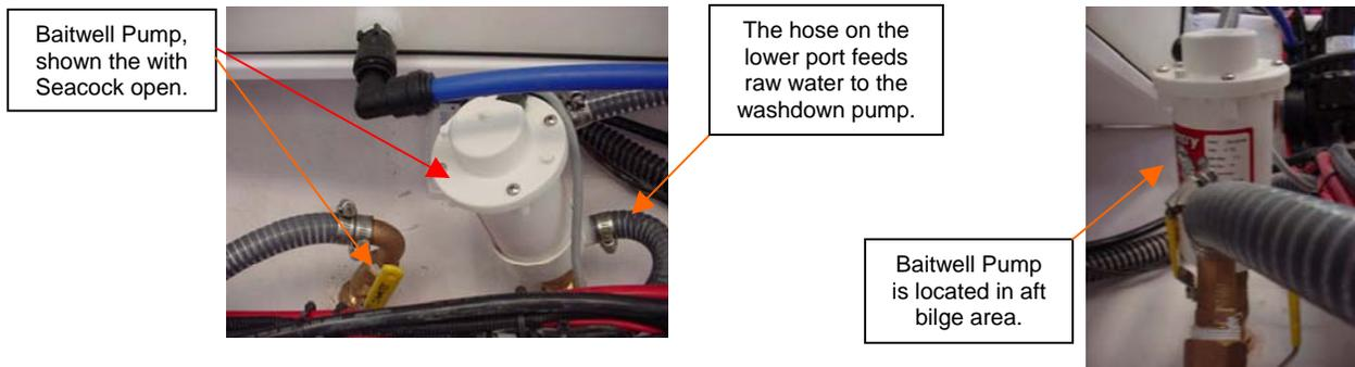
To operate the baitwell pump, locate the baitwell switch on the console and press the switch to the forward position to turn on the pump. When the baitwell pump is operating, go to the baitwell tub and visually check to see if water is pumping into the tub through the aerator fitting. This will ensure that the baitwell pump is working properly.
