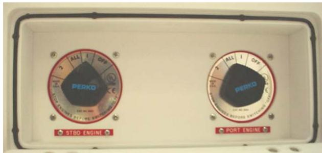
**Caution:** To avoid possible alternator/battery damage on twin-engine installations, make sure that the dual battery switches are never left so both engines are connected together, (i.e., never leave a switch on "BOTH" or "ALL"). The preferred switch position is port engine to position one (1) on the port battery switch and starboard engine to position two (2) on the starboard battery switch.
