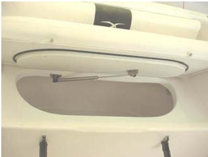
The 45-gallon capacity baitwell tub is located below the transom seat. It comes equipped with an aerator head, 2 overflow drains that allow circulation to keep bait alive, a plug for the drain and a baitwell light.
