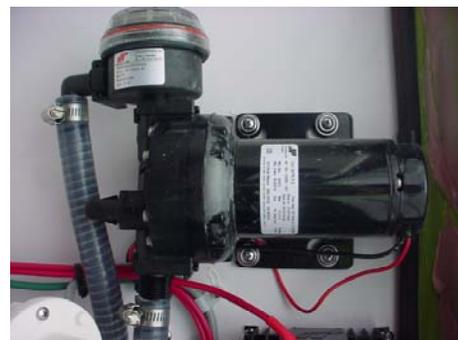
If the fresh water system is not in going to be in use, return to the switch panel and turn the cabin water system switch to the off position. When you close the faucet, the pump may run briefly. If the pump continues to run with the faucet closed, check the system for leaks or have the pump tested.
