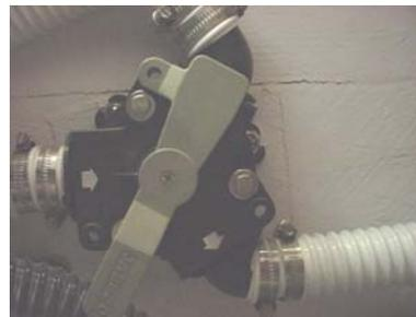
Then, go into the head area and flip the macerator switch to the on position.
