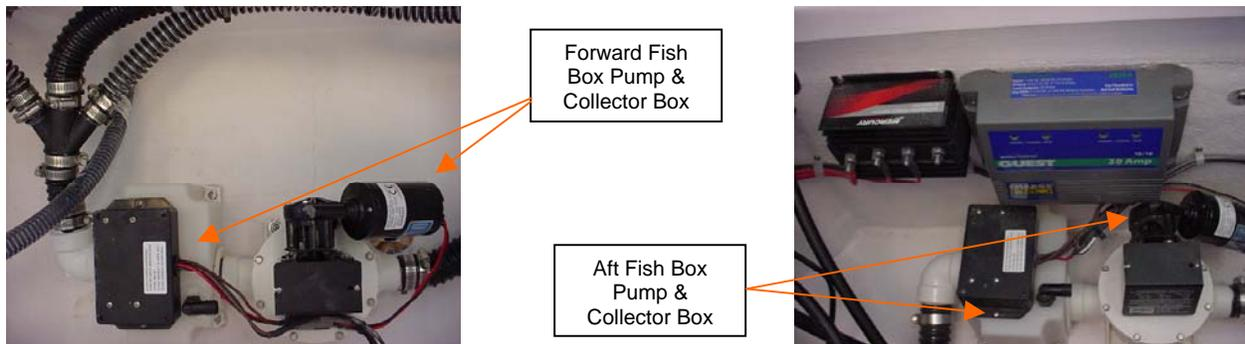
The fish box macerator pumps operate on separate 2-way rocker switches (labeled Fish Box) that are located on the switch panel.
