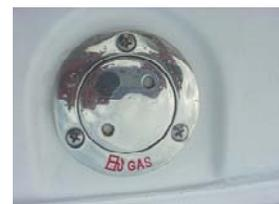
Note: Never pump fuel into any fitting, opening or access on the boat unless it is labeled "Gas" or "Fuel".
