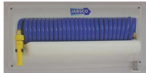
After checking for water and before returning the washdown hose to the storage compartment, turn off the washdown pump at the helm to release the water pressure in the hose. Twisting the hose clockwise allows you to easily stow the hose away.
