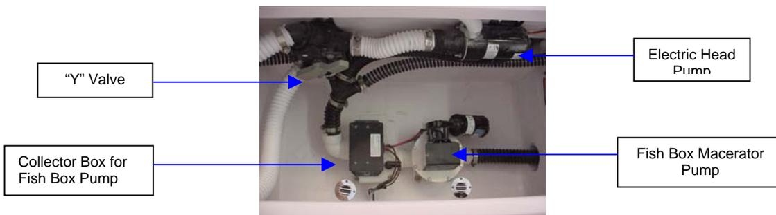
The “Y” valve is installed on the port side of the pump. It allows you to switch back and forth between dockside and overboard discharge. The photos below show the 2 positions for the “Y” valve (i.e., dockside discharge vs. overboard discharge).
