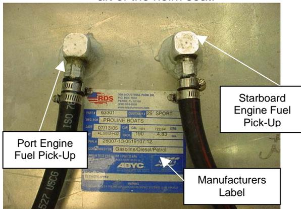
Located below the access pie installed forward of the helm seat and aft of the console.
