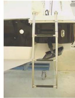
An optional dive ladder can be installed on the port side of the dive platform for additional boarding capability. When factory installed, this option includes the installation of an additional grab rail on the port transom. With the engines tilted down, passengers can move easily through the transom door and across the large dive platform to the optional ladder.
