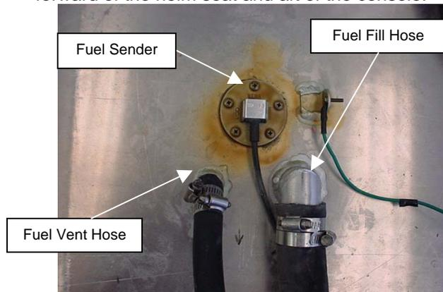
Inspect all hose connections on a regular basis. You can access other end of the fuel fill and fuel vent hoses via the 6" deck plate that is installed inside the compartment located starboard of the helm seat. This compartment also contains the washdown hose.
