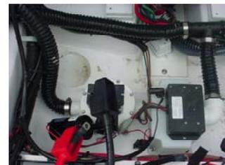
To activate the pump manually, depress the switch to the up or forward position. This action will drain the fish boxes of water and/or debris, transport it into the collector box/holding tank and then to the macerator pump to be macerated and/or discharged overboard.
