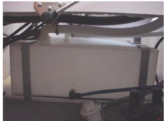
Important: Fill the tank with potable water only. Refilling the tank often will help to keep it a source of clean fresh drinking water. Never fill the fresh water tank with anything other than fresh water.
