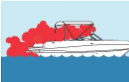
Exhaust gas trapped in enclosed places.
