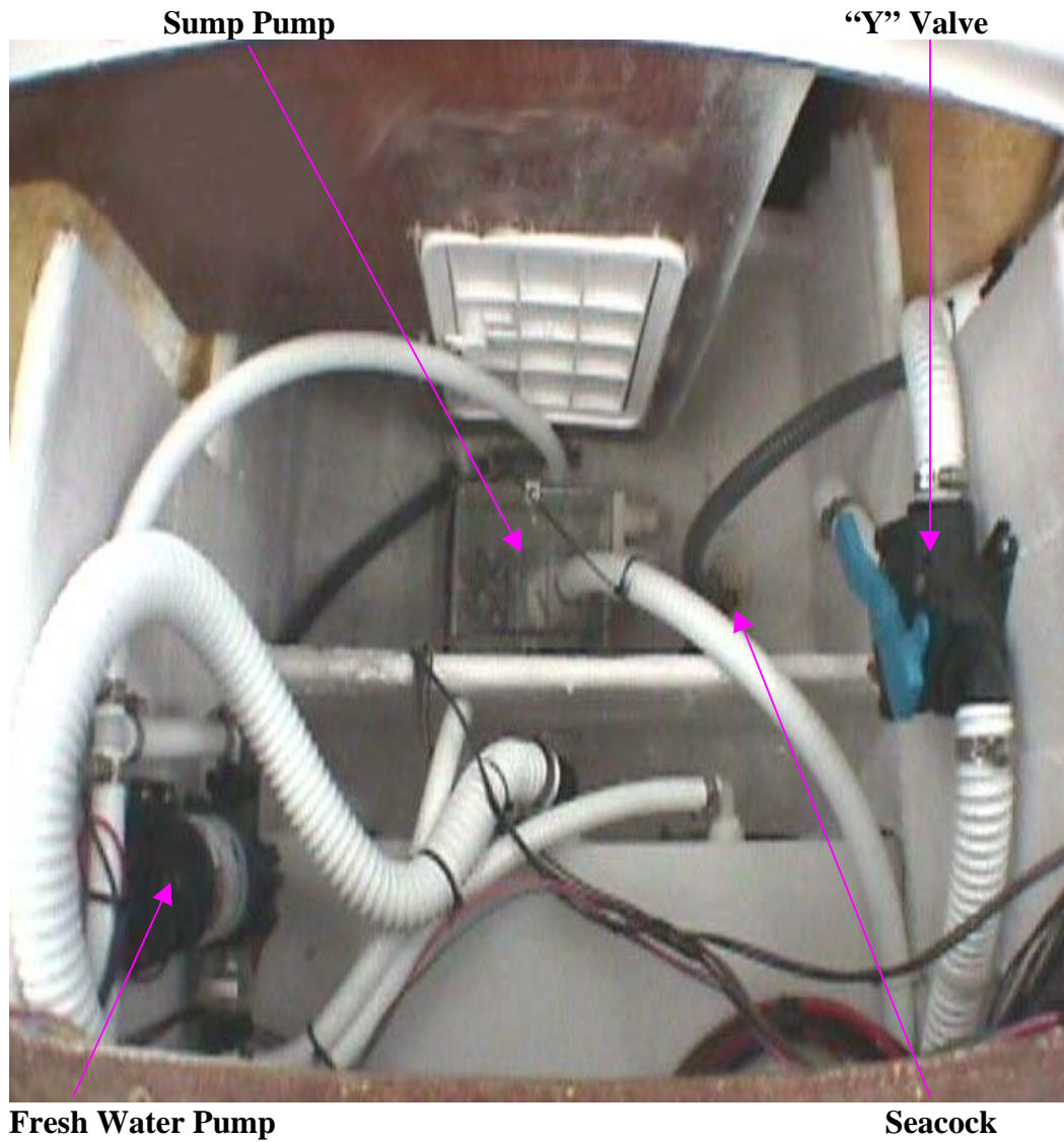
<fig. 9 – Head / Waste System>
