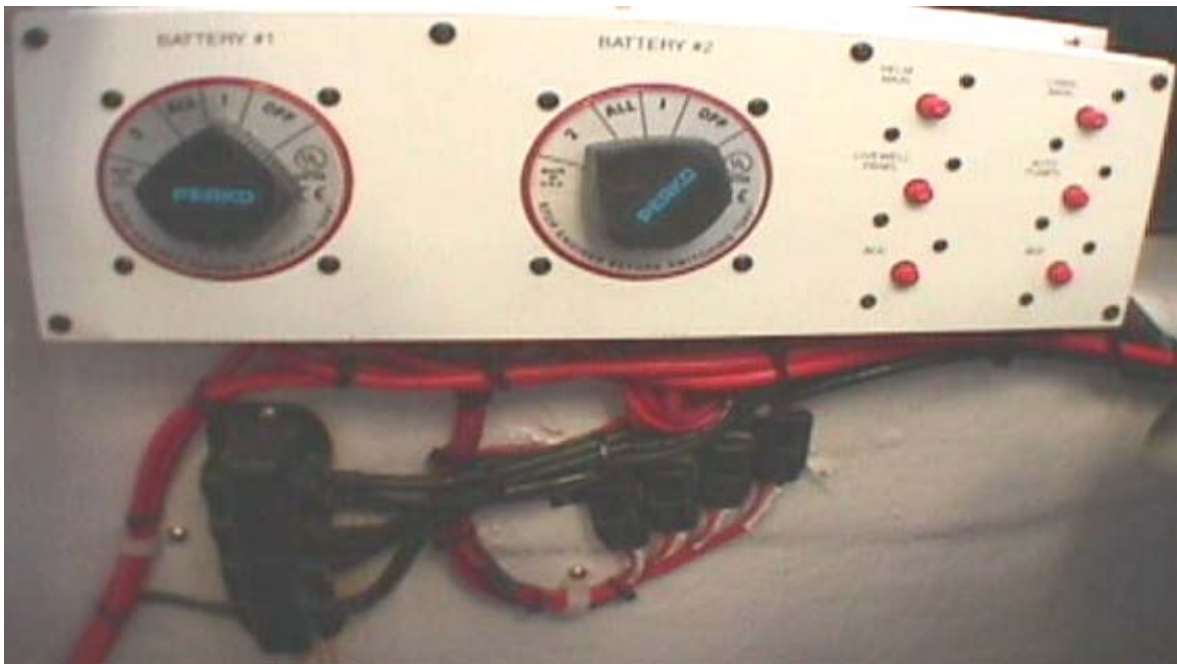
Bilge D/C Breaker Panel and Fuses
