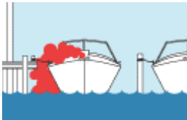
Blocked exhaust outlets.
