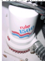
Bilge pump 2 (Bilge pump 1 is under the optional generator)
