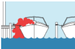
Blocked exhaust outlets.
