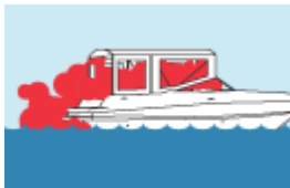
Inadequately ventilated canvas enclosures.
