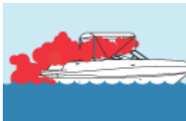
Exhaust gas trapped in enclosed places.
