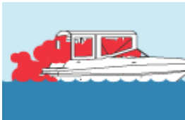
Inadequately ventilated canvas enclosures.
