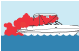
Exhaust gas trapped in enclosed places.
