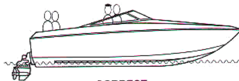
CORRECT Balanced load: gives maximum performance
