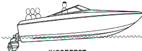
INCORRECT Overload aft: causes boat to "porpoise"
