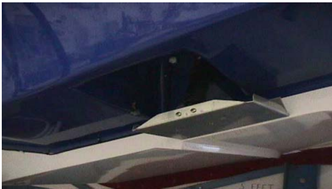
Fig. 3 trim tabs, shown in the up position
