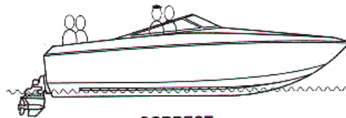
CORRECT Balanced load: gives maximum performance
