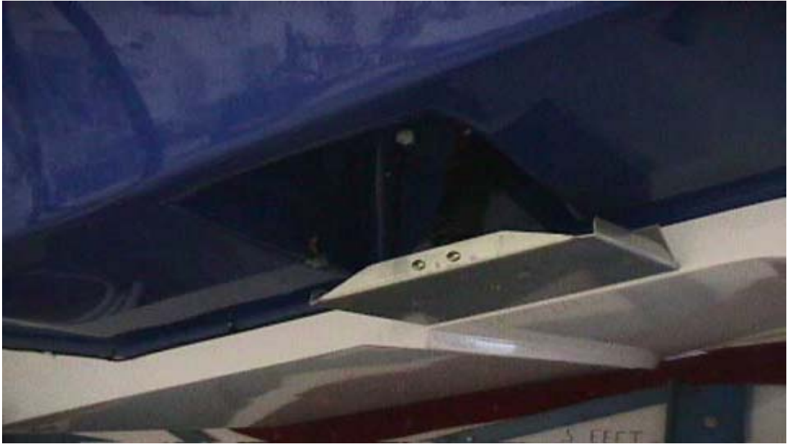
Fig. 3 trim tabs, shown in the up position
