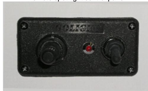
Remote spot light control panel
