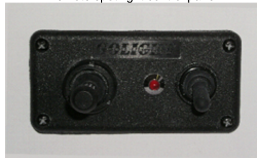
Remote spot light control panel
