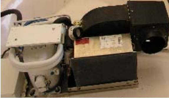
Air Conditioning Unit – Under the V-Berth
