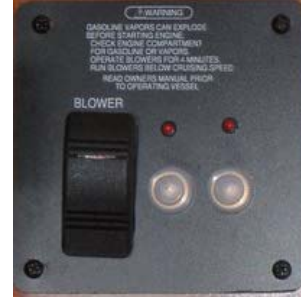
Blower Switch – Next to the AC/DC Panel
